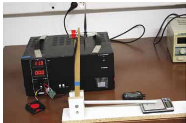
Fig.3 Experimental platform for measurement of thrust
