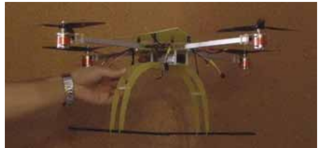
Fig.7 Position of quadrotor after rotation by an angle phi
